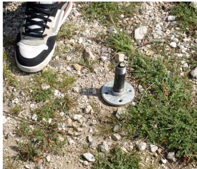
Figure 6. Rebar penetrated to standard depth.
