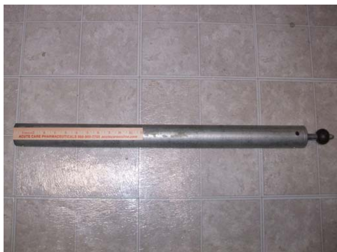
Figure 2. Sliding hammer in 2” diameter pipe.
