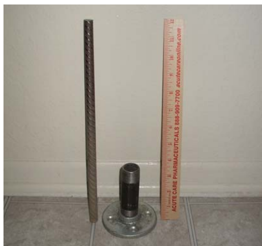
Figure 1. Penetrometer rebar and collar.
